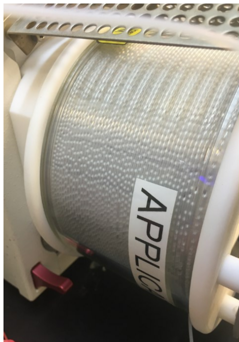
Figure 6: 1:1 Ratio of Gas:Liquid with Syrris Asia Reactors.
