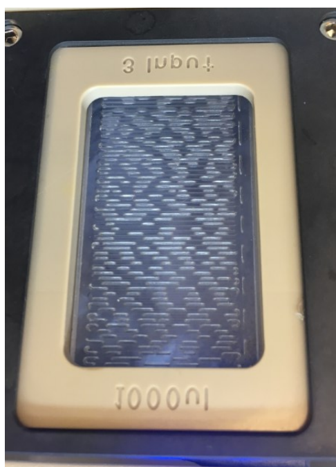
Figure 6: 1:1 Ratio of Gas:Liquid with Syrris Asia Reactors.
