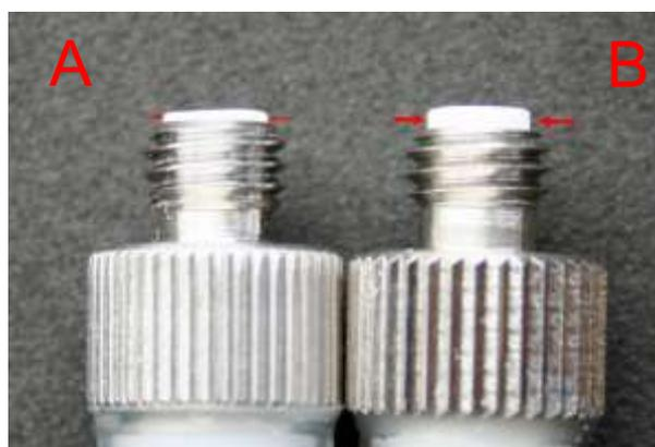
If the syringe has been worn (syringe A), a small PTFE washer may be inserted into the valve port, although it is recommended to purchase a replacement syringe at this point.
