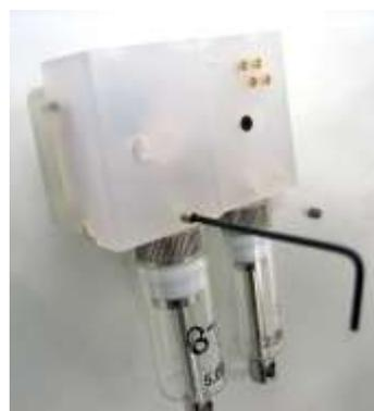
Use a metric 1.5mm Allen/Hex key to remove/loosen the grub screws. Under no circumstances, do not try to screw/unscrew syringes with the small grub screw in place. With the grub screws removed, the syringes should unscrew easily and can be removed. When inserting new syringes, please ensure to take care when screwing the syringe into the PCTFE valve to avoid cross-threading the valve. If any resistance is felt, remove the syringe and re-thread carefully.
