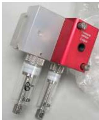
Unscrew and remove the pressure sensor. Take note of the grub screws which lock the syringe thread in place.
